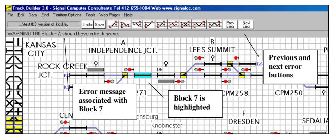
Figure 62 - Highlighted Track Elements
