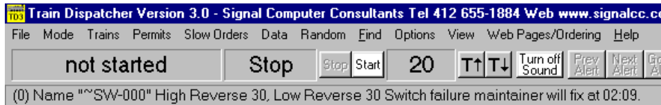
Figure 10 - Switch Status Line
